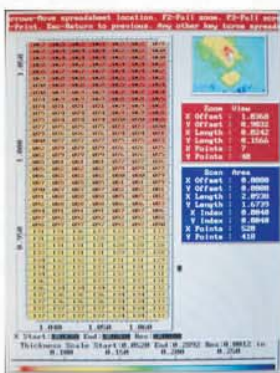
Zoom to Spreadsheet Mode of Corrosion Scan
